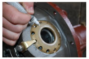
Figure 2 Mark carrier, caps & adjusters at lock hole.
