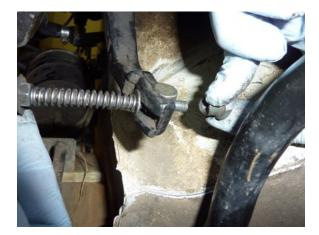
Step 3 Remove the cable adjustment nut.
