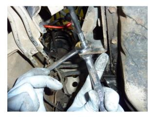
Step 24 Place the cable in the cable bracket and tighten the nuts using two 14mm open end wrenches.
