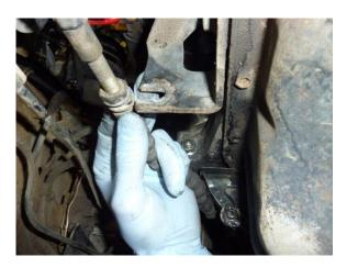
Step 7 Remove the clutch cable from he bracket.
