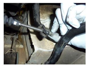
Step 22 Install the clutch adjustment nut.
