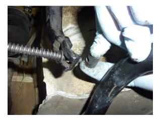
Step 4 Remove the clutch cable pivot.
