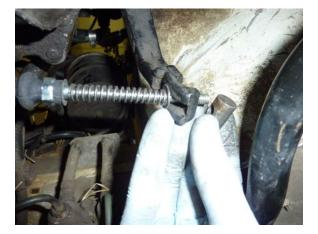
Step 21 Install the clutch pivot.
