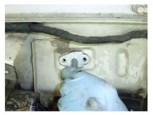
Step 18 Align the holes and install the grommet bolts.
