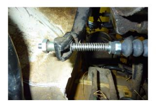
Photograph of Clutch Cable adjustment Nut
