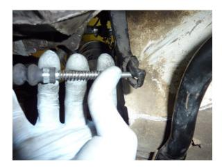
Step 20 Insert the cable through the clutch release arm.
