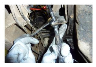
Photograph of Clutch Cable Bracket.
