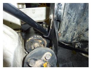
Step 15 Bend the cable restraint back as it was originally, securing the clutch cable.
