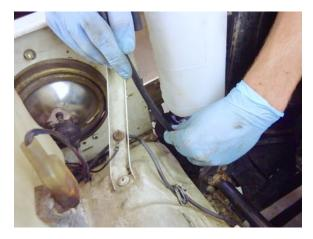
Step 12 Remove the clutch cable.
