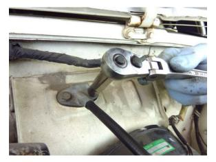
Step 9 Remove the clutch cable grommet bolts using a 10mm socket.
