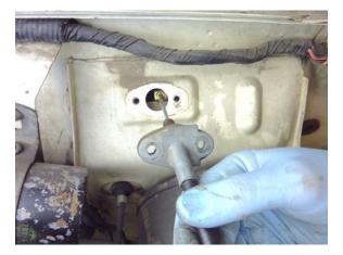
Step 10 Pull the clutch cable through the bulkhead.
