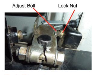
Tech Tip 26A This shows the pedal height lock nut and adjust bolt.
