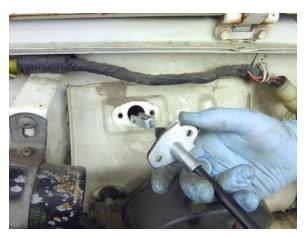
Step 16 Feed the new cable clevis through the bulkhead as shown.
