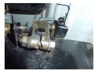
Step 17 Hook the clevis pin over the clutch pedal lever.
