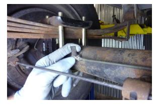
Step 2 Bend the brake line tab open.
