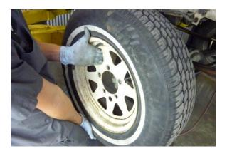
Replace both front wheel assemblies and tighten the lug nuts in a progressively tighter criss-cross pattern until 36.5 to 57.5 ft. lbs. is reached. Lower the vehicle to the floor.
