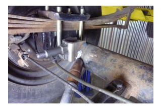
Once you are **<u>COMPLETELY</u>** satisfied that the mount is properly positioned, remove the lower end of the shock and weld the mount on both sides.
