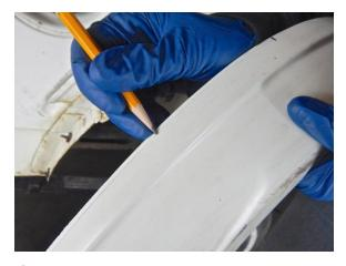
Using a pencil (or pen) make a line from the mark made in Step 7, 1/8 inch wide to the rear of the fender flare.
