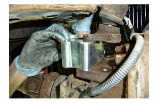
Step 5 Position the supplied spacer as shown and align the holes.
