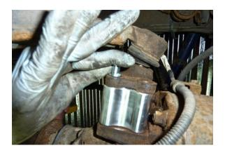
Step 6 Install the (4) supplied bolts and lock washers as shown.
