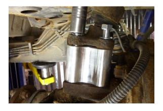
Step 7 Tighten the bolts using a 14 mm socket. (29 to 43 ft. lbs.)
