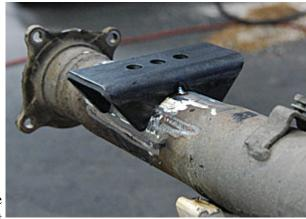
flange. Rotating the axle will shear perch the tack welds. Once the axle rotation has been chosen, re-tack perches in place.
