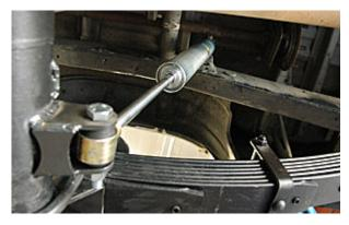
For best results use the RTI ramp or forklift to twist the rear suspension and verify the shock mounting positions. The shocks should be mounted in such a way they neither limit extension or compress the travel of the suspension. If this is not done, shock damage **will** occur. Shocks damaged by excess compression or extension, **are not** covered by warranty.
