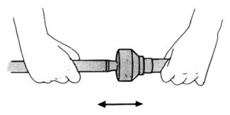
Caution: The axle shaft should only be installed into the birfield far enough to engage the snap ring into the groove in the birfield star. Over-inserting the axle shaft into the birfield will cause insufficient engagement on the differential side, which may cause the splines to fail. Failures caused by improper installation are not covered under warranty.
